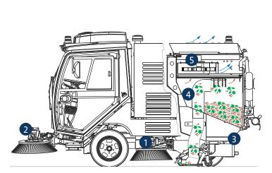
Debris are collected into the hopper by mean of suction without passing through the fan.
